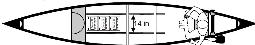
20-Ft Canoe using a 36V Motor. Batteries aft keep bow high with 2 people in boat:
