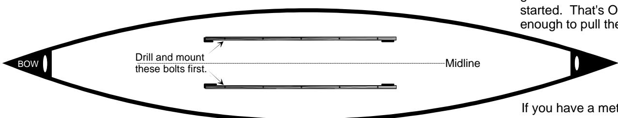
You might need to leave off the gasket or washer to get the nut started. That's OK. Tighten it enough to pull the bolt up.
