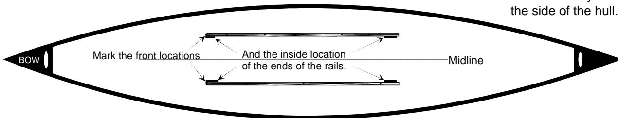
Note that the Rails are native hardwood, and may have slight curvatures. If so, place these curves so they match the curve of the side of the hull.
